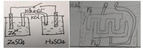
Figure 3-5 double fluid Cu-Zn- H<sub>2</sub>SO<sub>4</sub> voltaic cell
