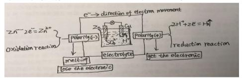
Figure 2-5 Cu-Zn-H<sub>2</sub>SO<sub>4</sub> voltaic cell (Level 4)
