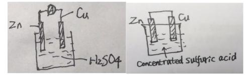
Figure 3-1 Cu-Zn-dilute H<sub>2</sub>SO<sub>4</sub> voltaic cell
