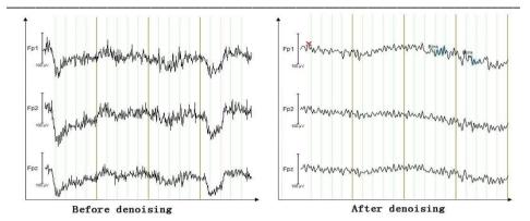
Figure 4. Comparison of before and after denoising of EEG signals collected by experiment
