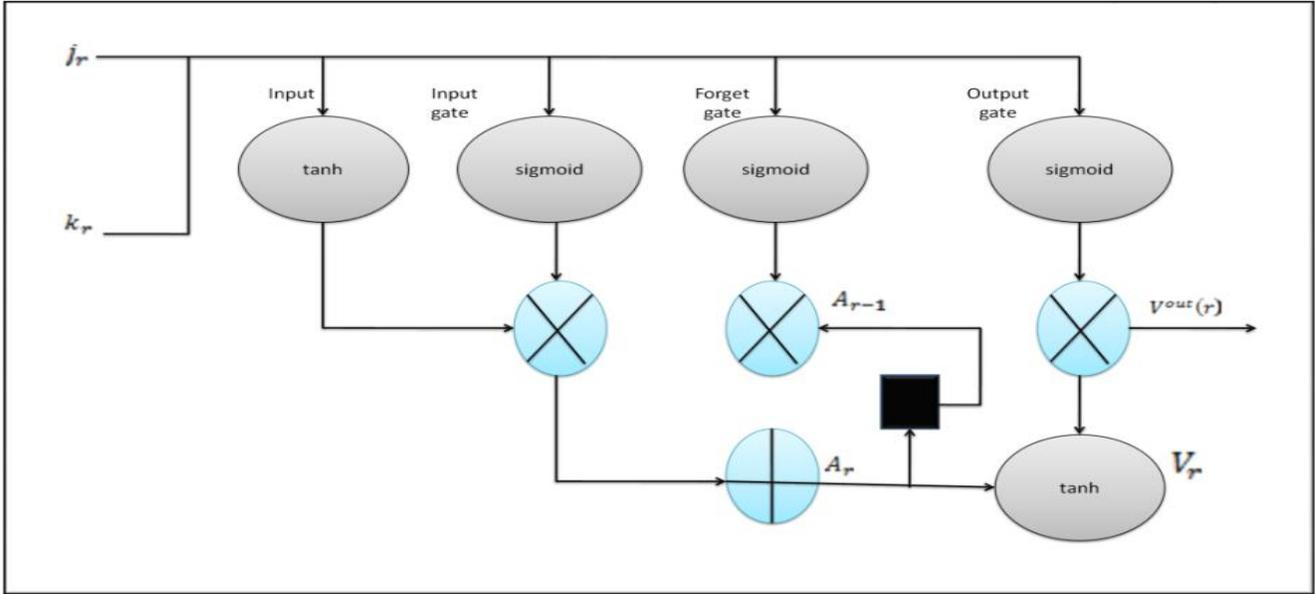
Figure 4. One cell in a basic LSTM network
